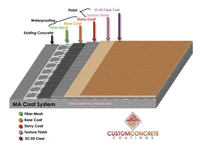
Ideal for areas with heavy foot traffic, Westcoat's MACoat is a fiber lath reinforced deck system engineered for use on elevated concrete and reinforced plywood walking decks. When sealed, MACoat offers a durable waterproof coating specified for use on balconies, corridors, stairs, plazas, and landings. Westcoat MACoat delivers superior durability and tough performance in hotels, condominiums, apartments, office buildings, and residential homes.
